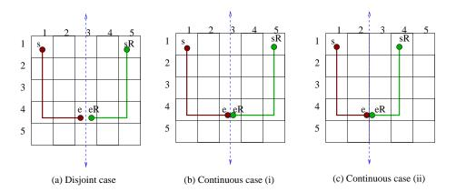
Figure 6: Disjoint and Continuous Cases. Symmetric strokes, consist of a defining stroke (solid line from s to e) and reflected stroke (solid line from  $s^R$  to  $e^R$ ). The last two, visually representing the letter 'U', show continuous cases where: (b) the axis cuts a set of cells; and (c) the axis is on a grid line.
